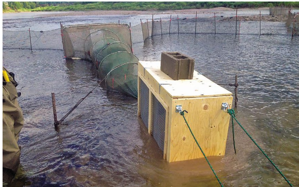
Fish trap being used by the Petitcodiac Watershed Alliance to monitor at-risk fish species. The box at the end of the net provides refuge from the currents, allowing the fish to rest and reduce stress. Species being monitored include striped bass, American eel and Atlantic salmon.
