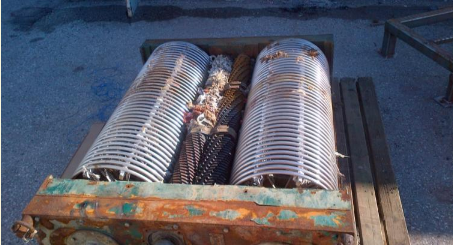
Grinder at pumping station.
